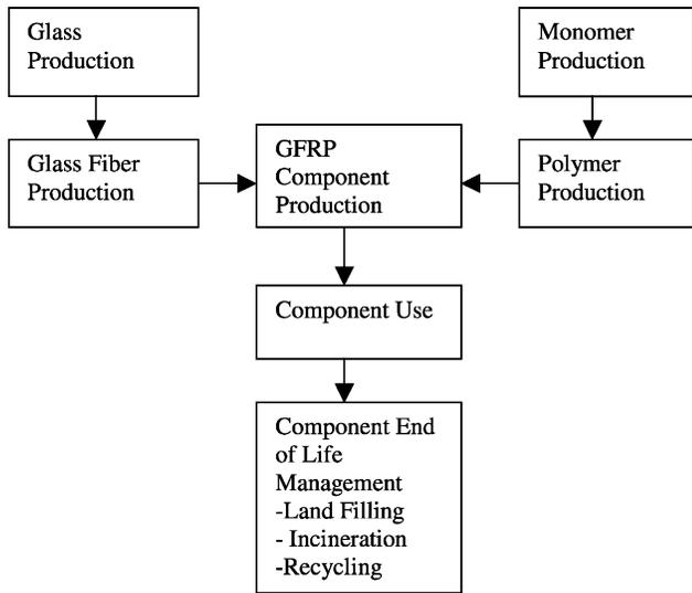
Fig. 1. Life cycle of a glass fiber reinforced composite component.
