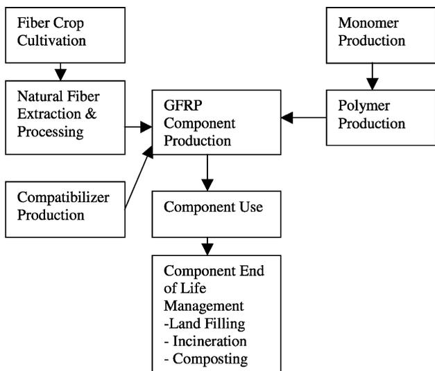
Fig. 2. Life cycle of a natural fiber reinforced composite component.
